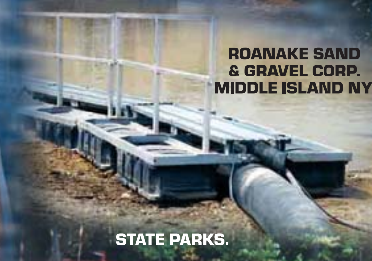
Floating removable DREDGING DOCK UNIT with walkway & handrail
